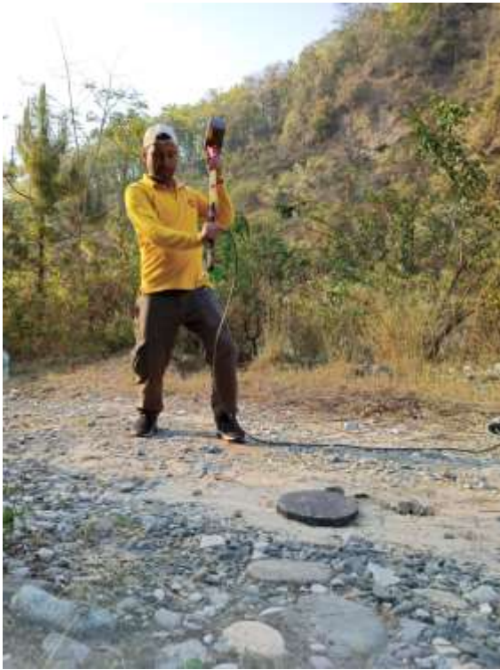
Sledge Hammer used as Seismic Source
