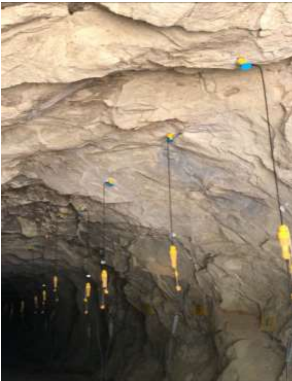
Placement of Geophones in Drift
